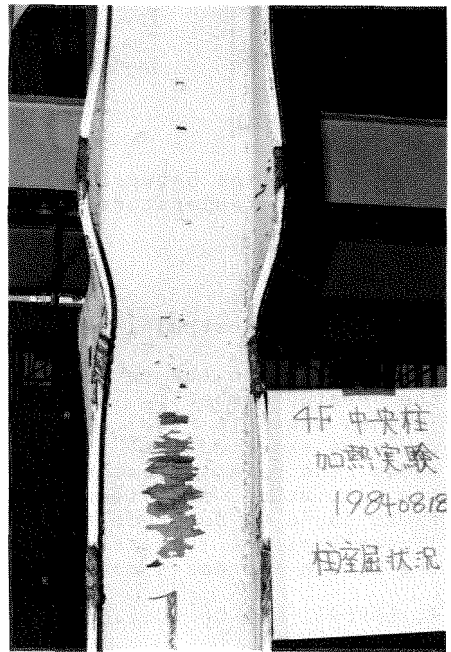
Photo.1 Local buckling of column ( K-1 )
