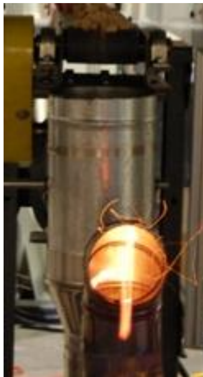
Fig. 3. Image of firebrands shower at exit of device.
