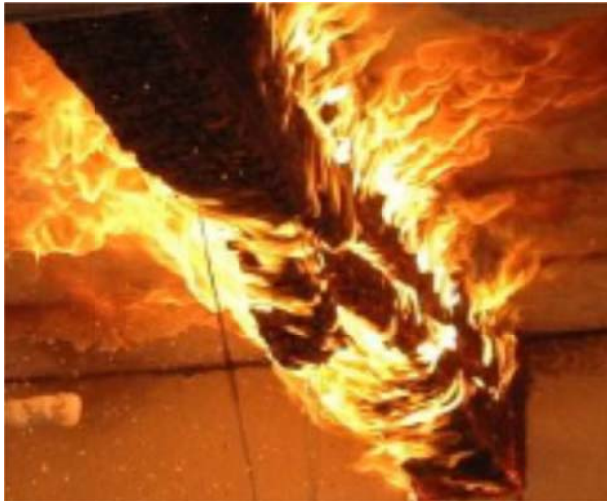
Fig 1. A timber beam during fire exposure. [4]
