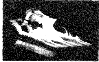
FIGURE 4. A photograph representing a typical aspect of the flame spreading in an air stream; T_i=20^\circ\text{C} , U=150 cm/s, x_1=15 cm ( x_1 -location of the leading flame edge).
