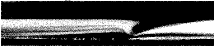
(c) Smoke streaks and leading flame edge ( t=0.25 s).
