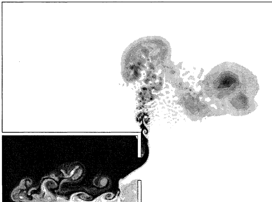
FIGURE 3: The mixing of hot (black) and fresh (white) air after the opening of a window. The grid size is 768 \times 192 cells, and the Reynolds number is 30,000.
