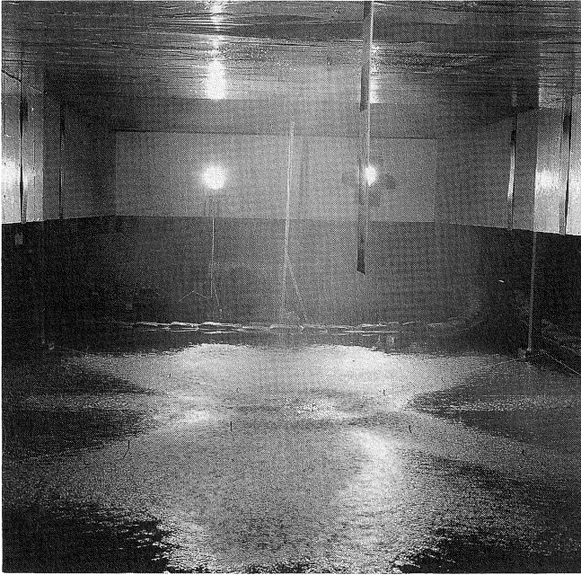
Figure 1 Experimentally observed water splash pattern at floor for Wormald 'A' cu/p sprinkler – pendant position, 15mm bore, flow rate of 1 litre/s
