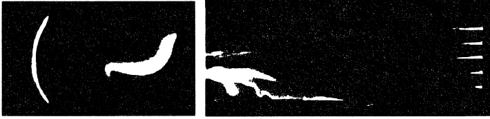
FIGURE 7 Top view of flame spread across an 80 mm wide by 2 mm deep pool of 1-butanol. (a) 1g: Smoke lines indicate flow pattern 1 mm above surface. Free-stream flow is left-to-right at 30 cm/s, while spread is right-to-left. (b) \mu\text{g} : flame is more erratic in shape, direction, and brightness. Curved bright line on right is a glowing igniter wire.
