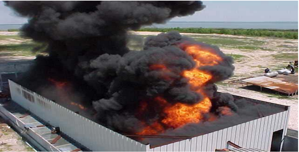
Fig. 3 Free-burn fire progress in Test 7. Fire intensity increased over time. This photo was taken 5 s before the water discharge.
