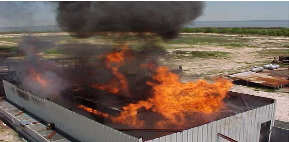
Fig. 4 Fire flare-up due to flame/water reaction in Test 7.
