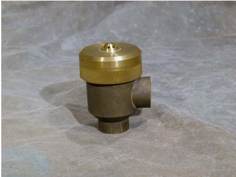
Figure. 3 The nozzle housing for the 10JET90 and 12JET90 nozzles.
