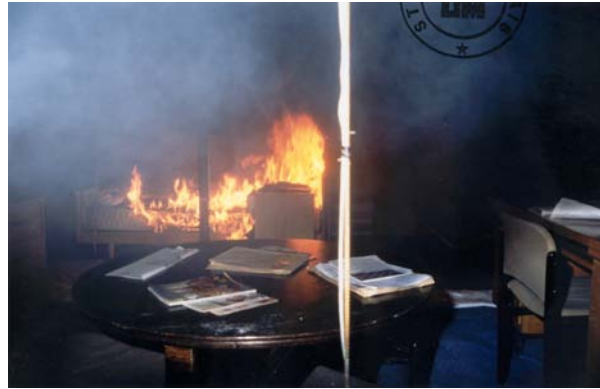
Fig. 4. Beginning of the fire by ignition of the mattress.
