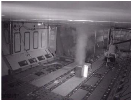
Fig. 3. Smoke generator test in an A340-600 aircraft.
