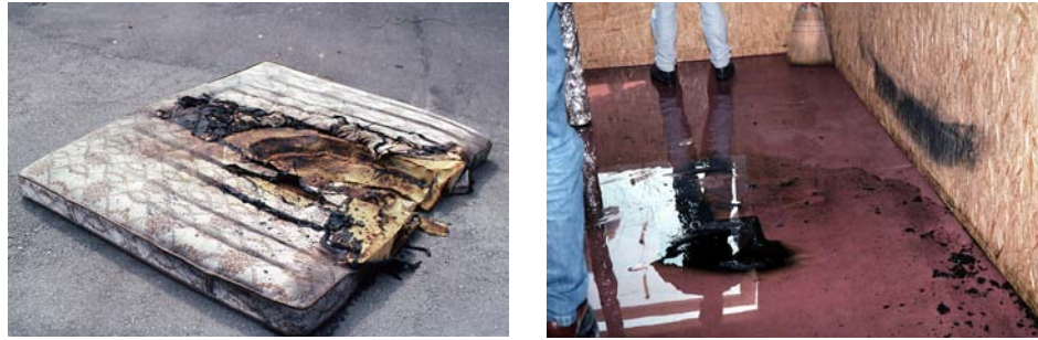
Fig. 4. Damages on the mattress (left) and on the wall and the floor (right).
