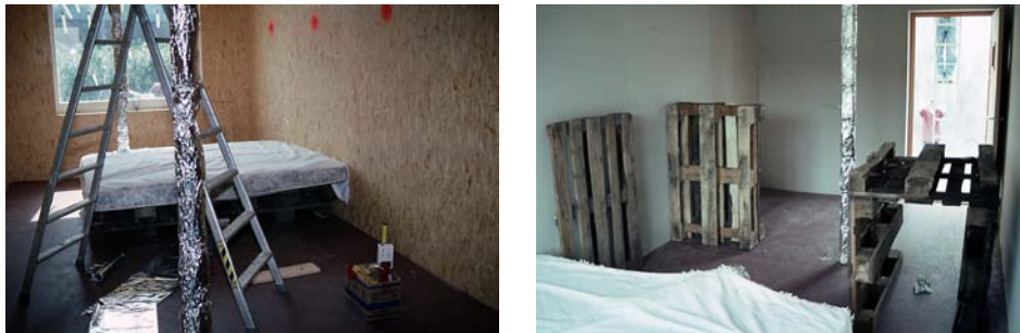
Fig. 2. Movable fire load consisting of a mattress (left) and wooden pallets (right).
