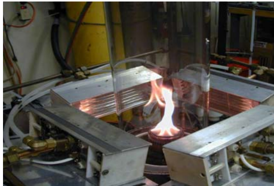
Fig. 2. Combustion section of the fire propagation apparatus (FPA).
