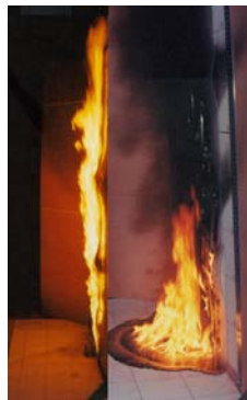
Fig. 2. Melting behaviors of PMMA (left) and PP (right) sheets installed in vertical orientation in large scale burn tests.
