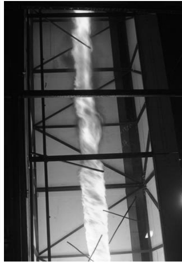
Fig. 5. Firewhirl experiment at SKLFS. The enclosure: 15 m high; firewhirl: 9 m high.
