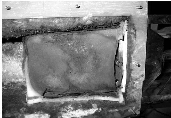
Fig. 2. Foam sample after smoldering process.
