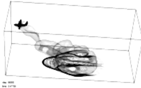
Fig. 8. Simulated area of water dropped from a flying boat for Case 1, where the numerical domain is enlarged.
