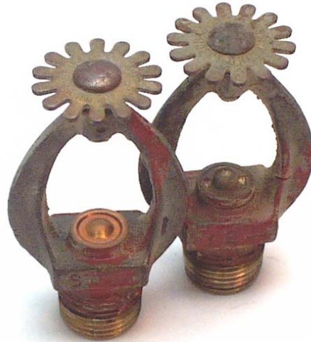
Figure 6. Examples of painted sprinkler heads
