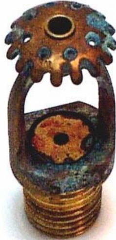
Fig. 5. Typical example of severe orifice seal corrosion of the sprinkler head.
