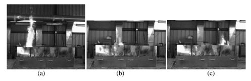
Fig. 3. Images of fire captured from videotape at time (a) t=60 s, (b) t=178 s, and (c) t=597 s, after the initial ignition with zero slope.
