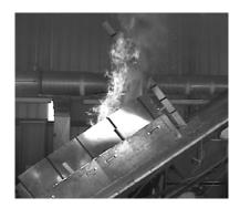
Fig. 5. Illustration of a fire image with the slope setup A of 70%.
