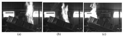
Fig. 6. Images of fire captured from videotape at time (a) t=19 s, (b) t=68 s and (c) t=176 s, after the initial ignition with the redesigned slope setup C of 40%.
