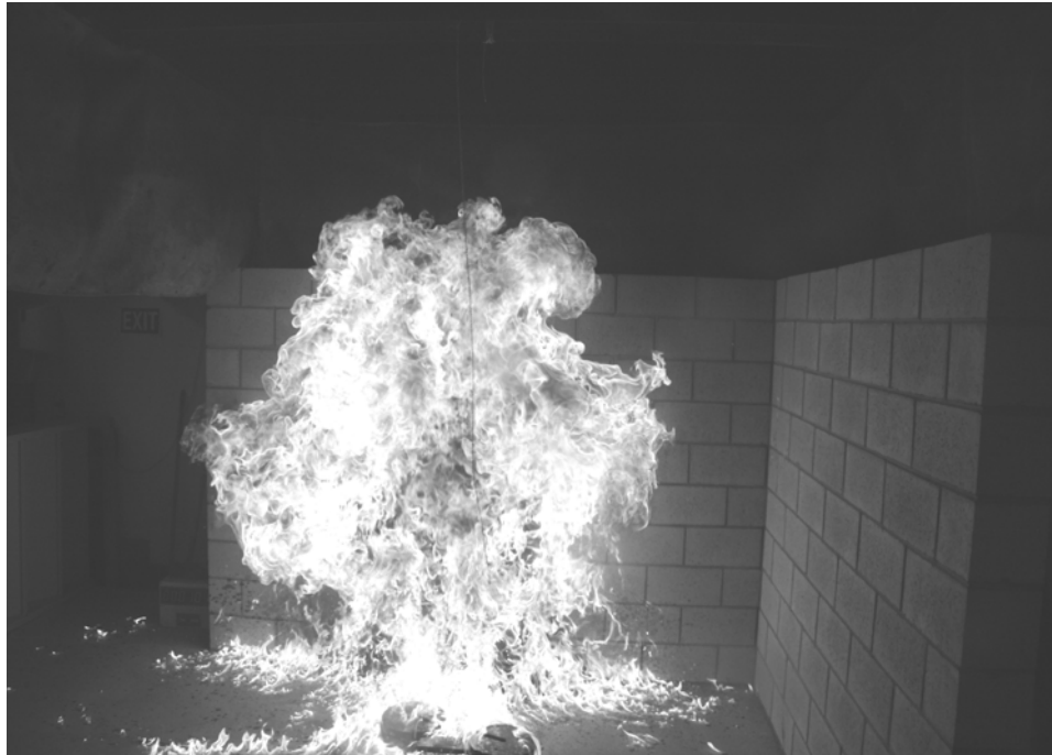
Fig. 2. Photograph showing the fireball immediately after the 1000 ml glass bottle full of common petrol strikes the electric knife blade igniter.
