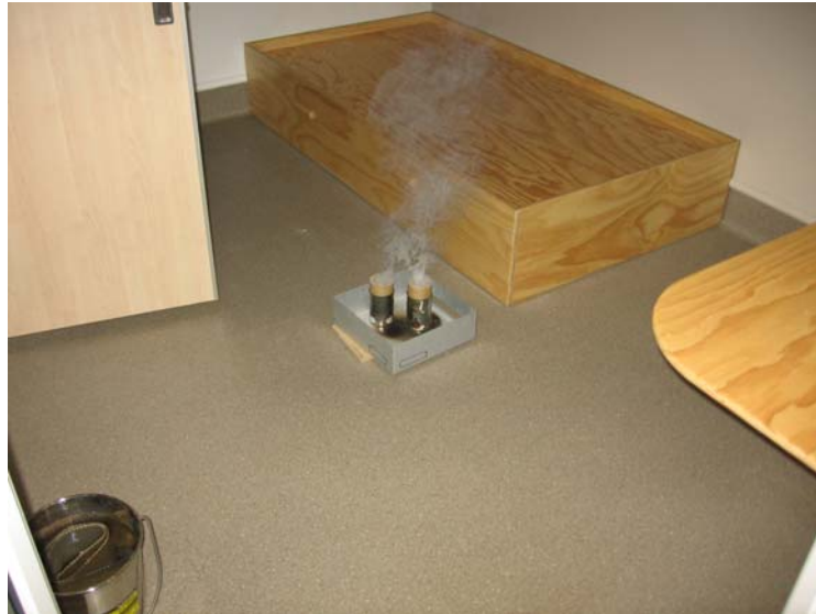
Fig. 5. Smouldering fire with rolled cardboard.
