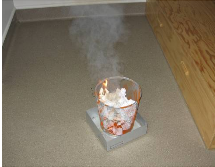
Fig. 6. Flaming fire with paper in bedroom.
