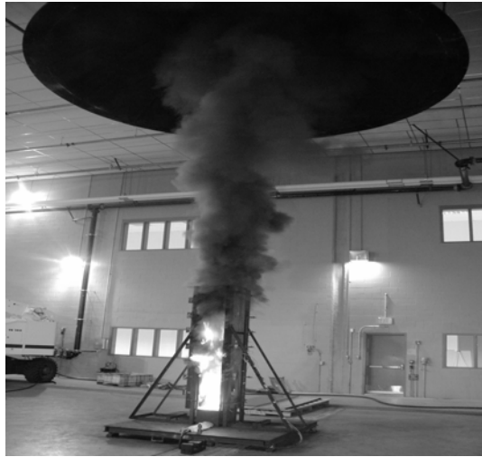
Fig 4. Two 4.9-m x 1.1-m PVC panels with a heat exposure of 360 kW from a propane burner under the 5-MW FPC. Figure is taken from Ref. 13.
