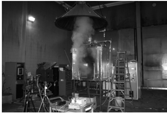
Fig. 2. A photographic illustration of the experimental setup of the Scale-1 enclosure and the 200-kW fire products collector.
