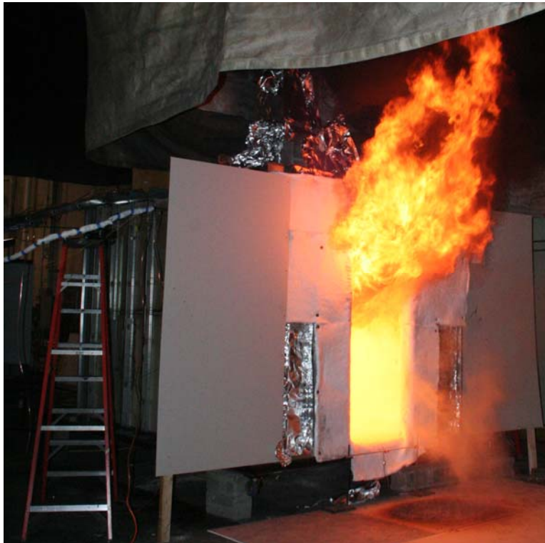
Fig. 2. Image of a 2.7 MW natural gas fire in the full-scale enclosure.
