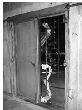
Fig. 7. Photograph of the doorway velocity probes for the 2-rooms configuration
